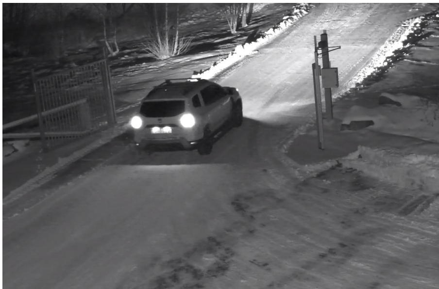
Figure 2-6 Overexposure of license plates
