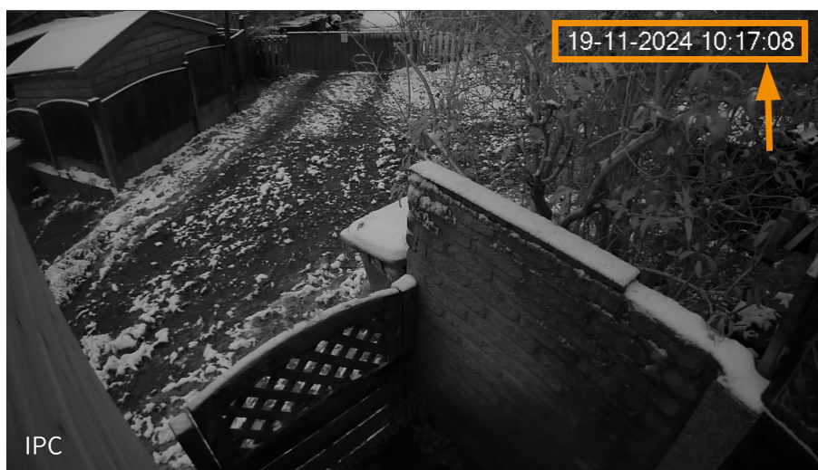
Figure 2-9 Day/Night mode failure
