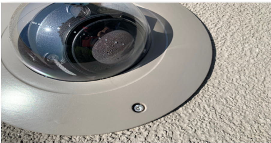
Figure 1-6 Moisture inside the camera
